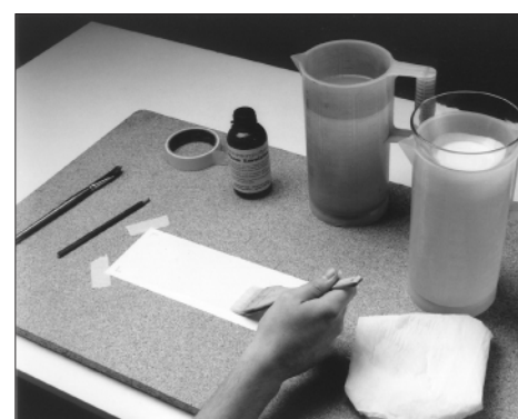
B. Producing test strips using the same materials and coating techniques as the full sheets
