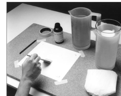
E. Emulsion being applied with vertical strokes
