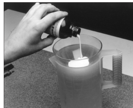
A. Emulsion held in a bowl over a jug of hot water.
